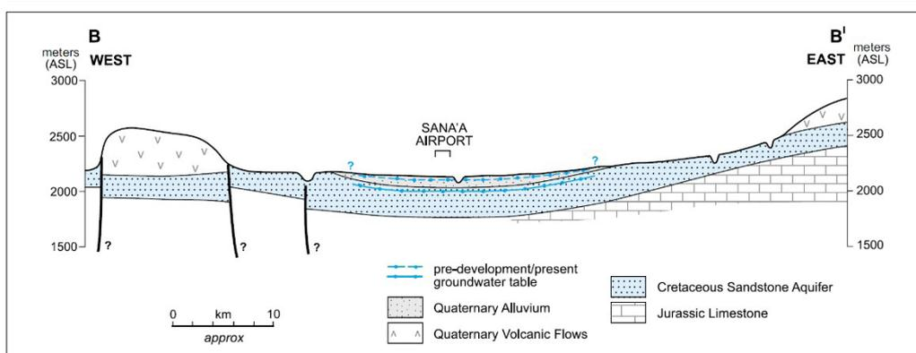
Figure 3: Hydrogeological map and cross-section (B-B) of the Sana'a Basin<sup>[44]</sup>
